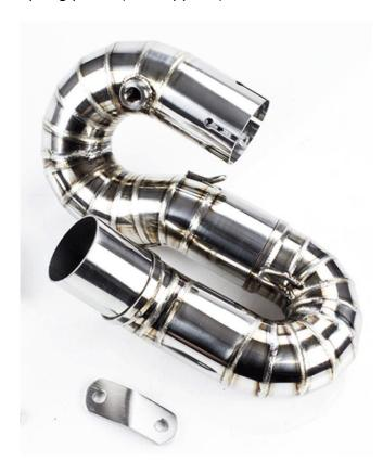
Add the clamp to the slotted end of the link pipe and apply a small amount of paste to the joint and allow to cure. Re-install the lambda sensor and tighten to 30Nm. Only finger tighten the clamp at this stage.
