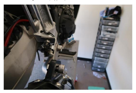
Mount your new Lextek Silencer to the downpipe and line the mounting point on the silencer to bracket (installed earlier). Secure the silencer using the clamp to a torque of 12Nm.
